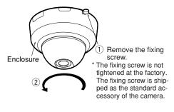
2. Detach the dome cover and the inner dome from the camera.
